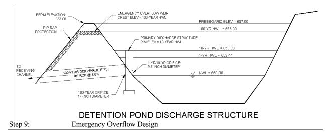
The emergency overflow device must be capable of conveying discharge from the 100-year fullydeveloped discharge rate. The HEC-HMS model indicates that the developed 40-acre parcel will discharge at a rate of 224 cfs (NRCS Type II 24-hour rainfall). The most practical way of providing an emergency overflow device for this flow rate is to construct a depression in the detention pond berm (overflow weir).
