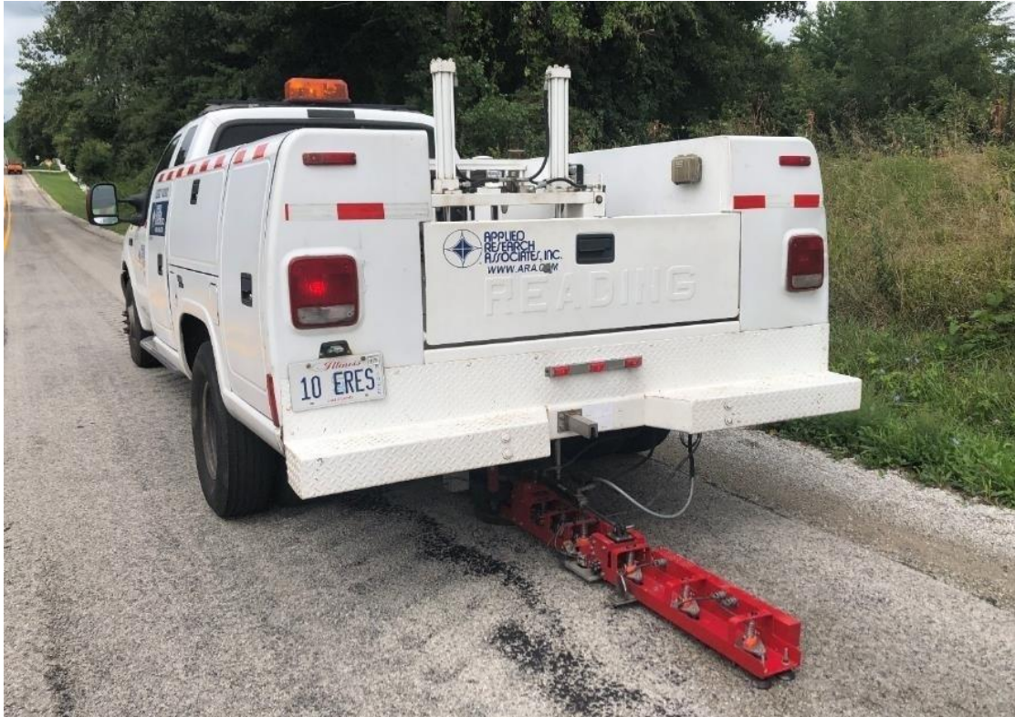
Figure 7. The FWD is a nondestructive testing measuring the pavement's structural response.
