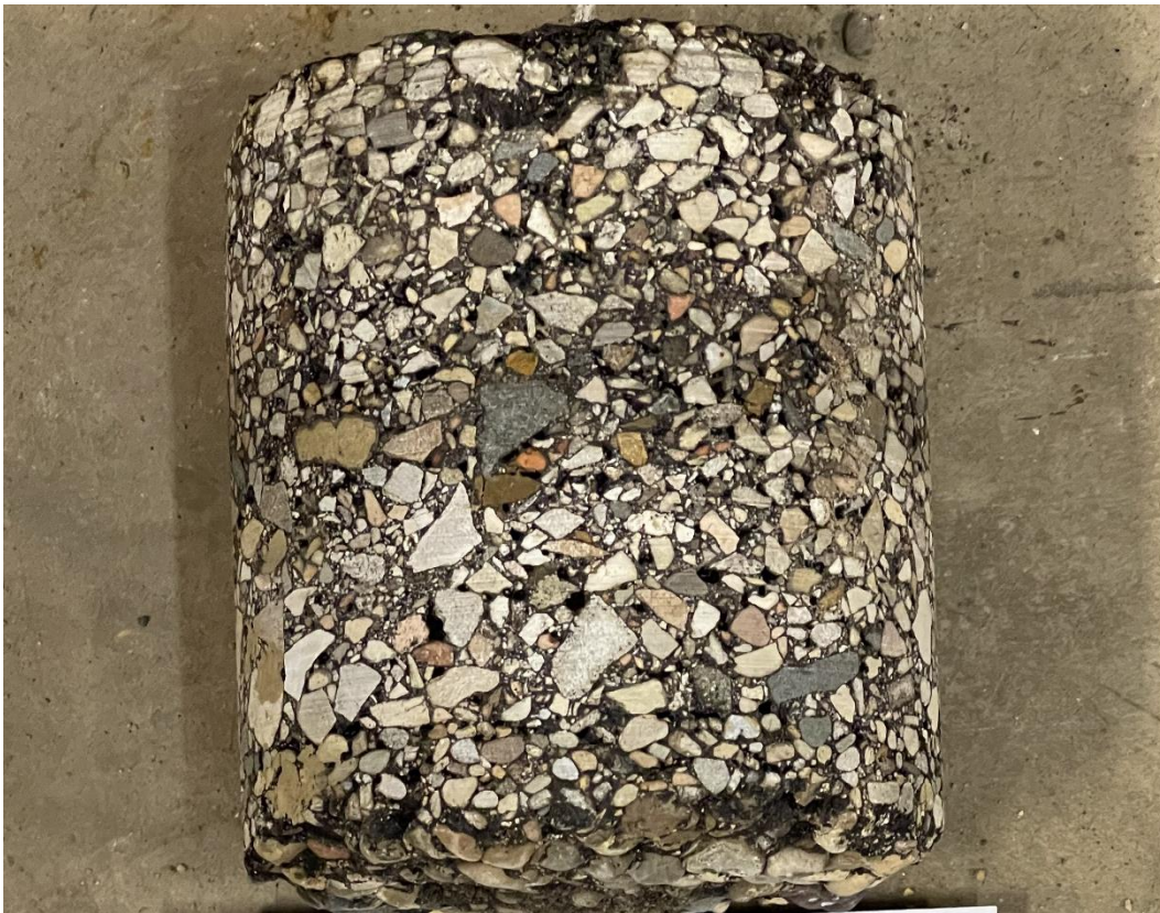
Figure 5. Combination of chip seal and AC layers – CH 25, mile 2.56.
