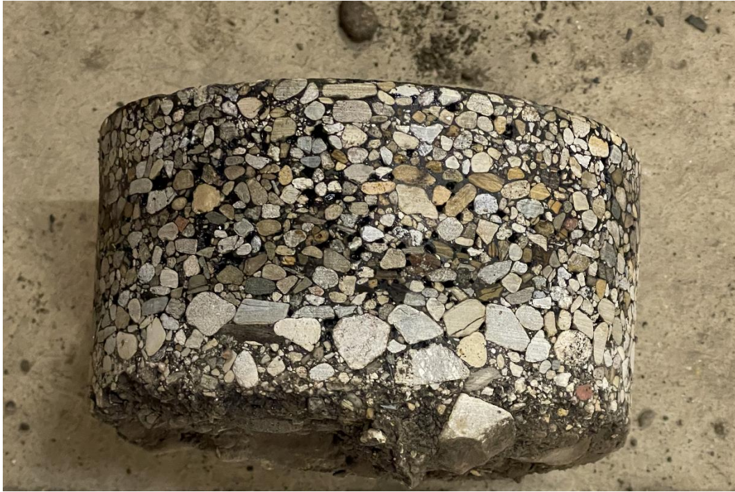
Figure 4. Typical core sample showing accumulated chip seal layers – CH 2, mile 0.5.
