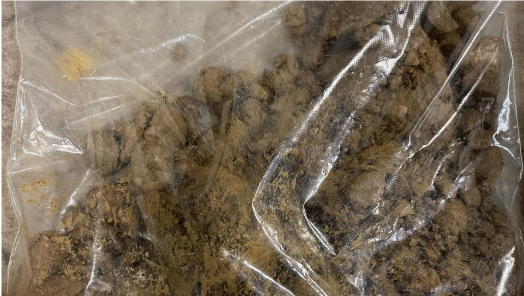
Figure 6. Sample crushed gravel with sand base – CH 3, mile 4.5.
