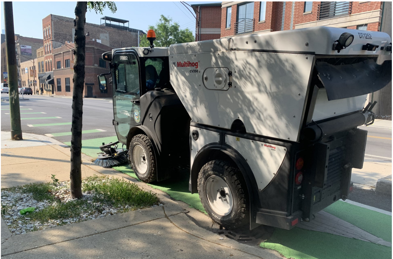
With its narrow profile, CDOT's Multihog maintenance vehicle can sweep and plow the City's separated bike lanes. (Source: CDOT)
