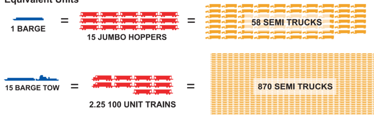
Figure F-7 Number of units needed to transport cargo via truck, rail, and barge (USACE, n.d.)
