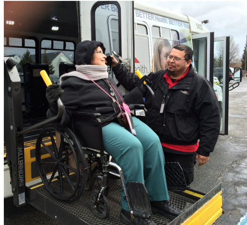
Figure 71. Driver assisting woman on wheelchair on lift. Photo credit: Senor Transportation Connection, Cleveland, OH
