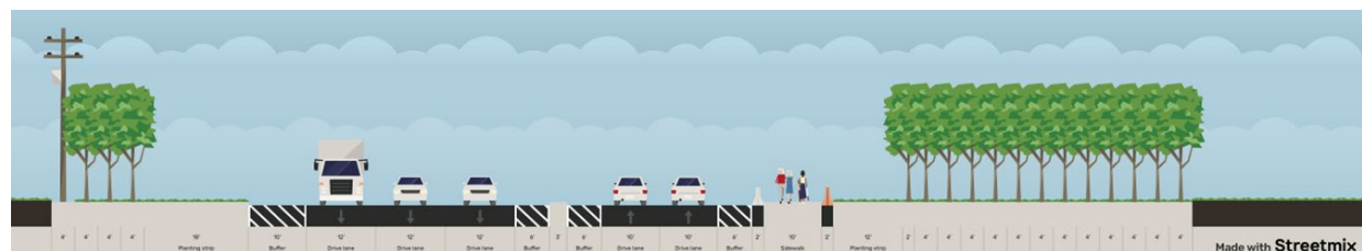
Figure 12: IL-116 looking SW at Byerly Hills Dr (alternate proposed approximate cross-section with roadway shoulders narrowed and WB lanes shifted east)
