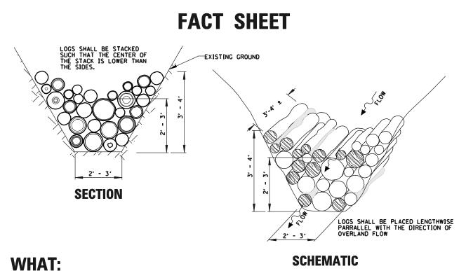
Small stack of logs placed in zero order or first order drainage ways that carry surface water flow only after storm events or snow melt.
